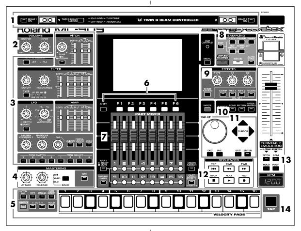
When you press the Mode section **[PATCH/SAMPLE] button**, the button's indicator will light and the MC-909 will be in Patch/Sample mode.
